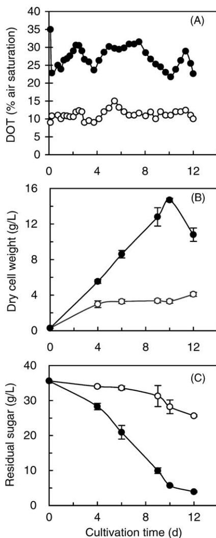
Fig. 5. Time courses of DOT (A), DW (B) and residual sugar concentration (C) during the submerged fermentation of *G. lucidum* in a turbine-agitated bioreactor. Symbols for DOT:  $\sim 10\%$  of air saturation ( $\circ$ ) and  $\sim 25\%$  of air saturation ( $\bullet$ ). The error bars in the figure indicate maximum errors from two independent samples of two reactors.
