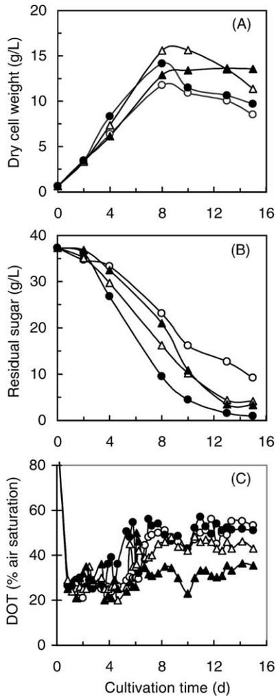
Fig. 1. Time profiles of DW (A), residual sugar concentration (B), and DOT (C) during submerged fermentation of *G. lucidum* at various initial  $K_{La}$  levels in a turbine-agitated bioreactor. Symbols for initial  $K_{La}$  values ( $\text{h}^{-1}$ ): 16.4 (○), 60.0 (●), 78.2 (△) and 96.0 (▲).
